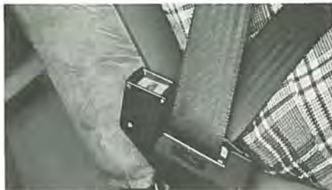
Front Belt in the Latched Position; upper part across chest, lower part across hips
