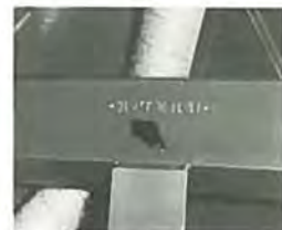
V.I.N. punched in car body, GLE, GL 5 door (under back seat cushion)
